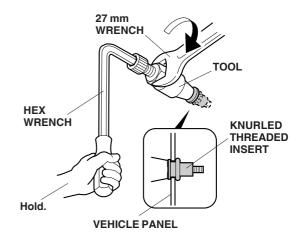
7. Remove the tool from the knurled threaded insert by turning the hex wrench counterclockwise.
