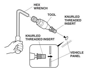
Holding the tool with the hex wrench, turn the 27 mm wrench clockwise to install the knurled threaded insert on the vehicle panel.
